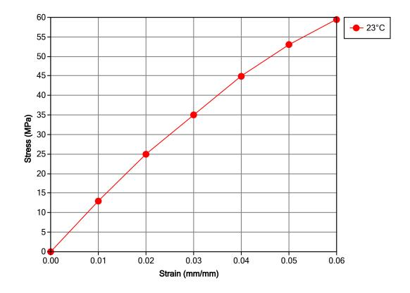
Secant Modulus vs. Strain (ISO 11403-1)
