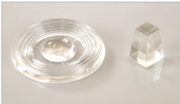
Optical LSR is a transparent, flexible thermoset material that is replacing glass in many optical applications.
