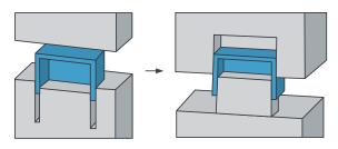
Using a core cavity, as shown, can be a cost-effective method of molding tall walls and ribbed surfaces.
