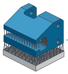
Support structures on DMLS parts help prevent curl that can occur during the sintering process. Read Full Cost-Saving Design Tips Online By Service
